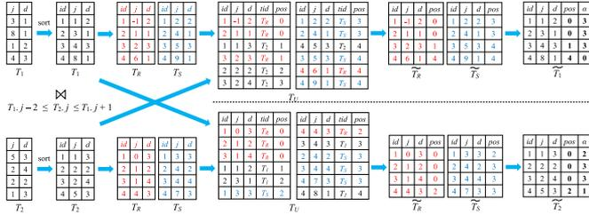
Fig. 2. Example of join degree computation.
